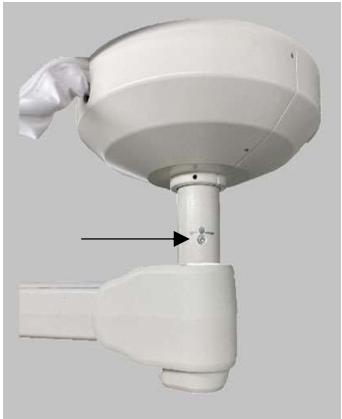
Figure 3 Correct: Mounting screw available and no visible damage
